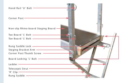
LSD STAGING BOARDS have a SAFE WORKING LOAD RATING OF 270KG in accordance with the requirements of BS 2037, evenly distributed over their length and are of welded aluminium construction. They are finished with "Rhino-board" boards with non-slip work surfaces and are produced in lengths of 2m/3m/4m/5m. The four metre and five metre boards have sockets on each side two metres from one end to accept our MID BOARD POST, which supports the handrails.
